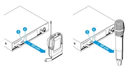
Press the synb button 3 on the receiver. "Sync" appears on the display panel of the receiver.
